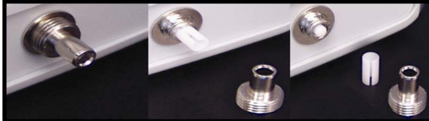
Fig 13.1 Split Sleeve Replacement
